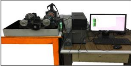
Fig 2: Configuration of data collection system
