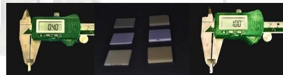
Two Teflon molds were fabricated with an external diameter of 20 mm×3 mm thickness, and the inner dimension 14×14 square shape was cut with two different thicknesses of 0.5 mm and 1.1 mm to accommodate the designated thicknesses of ceramic slices of 0.4 mm and 1.0 mm respectively and to ensure an 0.1 mm uniform thickness of resin cement samples.
