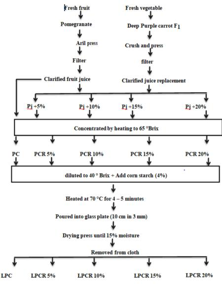
Fig. (1) Flow sheet for preparation of leathers
