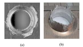
Figure 2. Photograph of a typical hole fabricated using friction stir drilling (a) top view and (b) bottom view.
