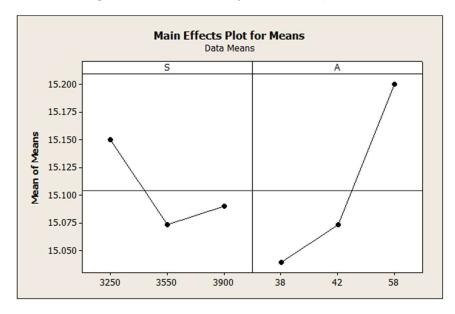
Figure 4. Main effects plot for means of the hole diameter.
