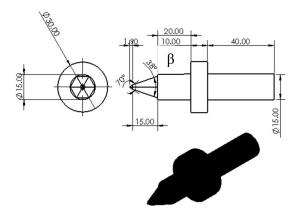
Figure 1. (a) The dimensions of the tool with hexagonal shape and conical angles ( $\beta$ ). The conical angle has values of 38°, 42° and 58°.
