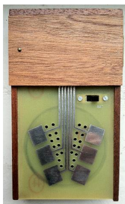
Figure 8 - A kraakdoos, a basic circuit bending instrument
