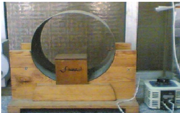
Fig. (1): The electromagnetic radiation exposure system was manufactured locally, in the Faculty of Science Cairo University.
