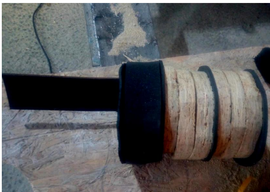
Fig. 5: Noise silencer for pipes with soundproof material.
