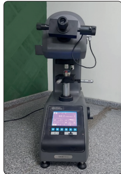
Fig. (1) Wilson microhardness tester.
