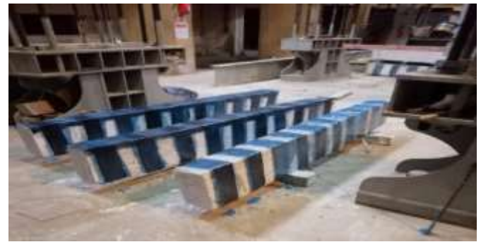
Figure 3: Beams with vertical CFRP sheets
