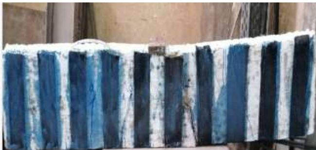
Figure 8: Tested RC beam (B2-1V-15) shear failure
