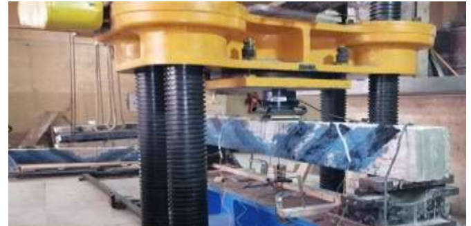
Figure 4: Beams with inclined CFRP sheets
