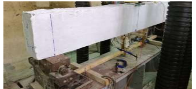
Figure 5: Control beam test
