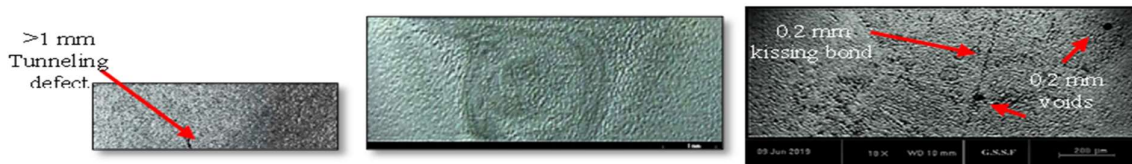
Fig. 3.8 Macro/Micrographs of the surface of friction stir welding sample for taper pin profile (run # 15).
