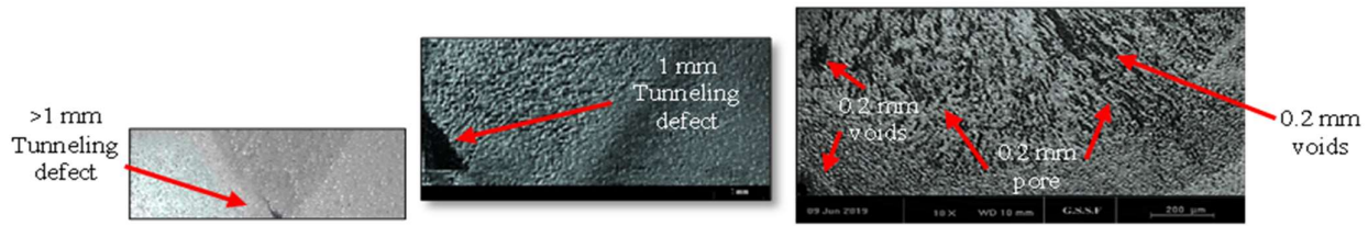
Fig. 3.5 Macro/Micrographs of the surface of friction stir welding sample for taper pin profile (run # 1).
