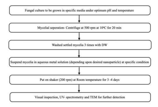
Fig. 4. Green synthesis of the NPs using the halophilic fungi (Huston et al., 2021)
