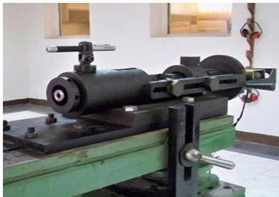
Fig. (3) HPI Ballistic rifle of caliber 9 mm and its mount
