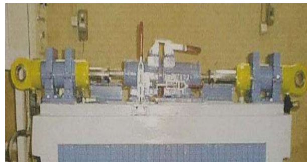
Figure 3-1 the real arrangement of the magneto abrasive flow machining process
