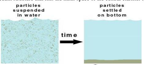
Fig 4 Sedimentation process<sup>(9)</sup>.
