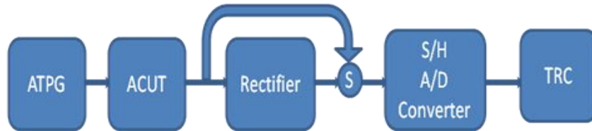
Fig. 2. Main block diagram of the presented analogue testing approach.
