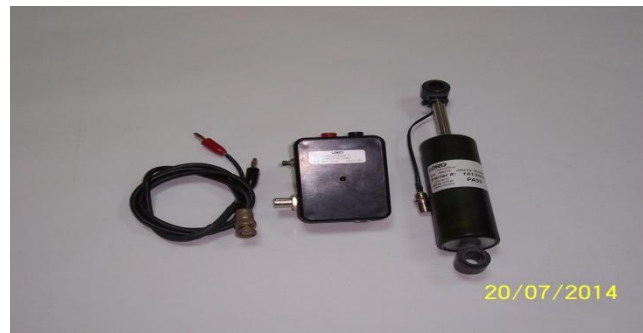
Fig. 3. MR fluid damper with control box and cables.
