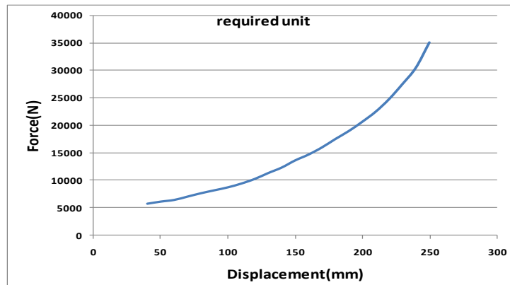
Fig. 10. Variation of HSU force at road wheel and corresponding vertical shift.
