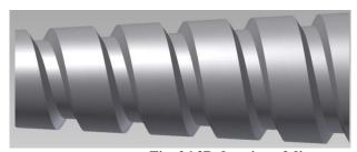
Fig. 26 3D drawing of divergent screw.
