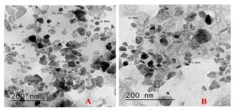
Figure. 3 The transmission electron microscopy (TEM) was performed for the synthesized nanoparticles at 200 nm. The size of the particles for CaNPs (A) is between 15.05 and 35.21 nm, while the size of CaNPs with oxalic acid is around 15.90 to 25.00 nm. The shape of the particles is spherical, and the small numbers are tetragonal. The particles in the case of CaNPs are more aggregated than CaNPs with oxalic acid particles (B).
