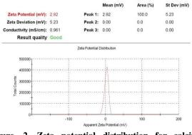
Figure. 2. Zeta potential distribution for calcium nanoparticles with oxalic synthesized
