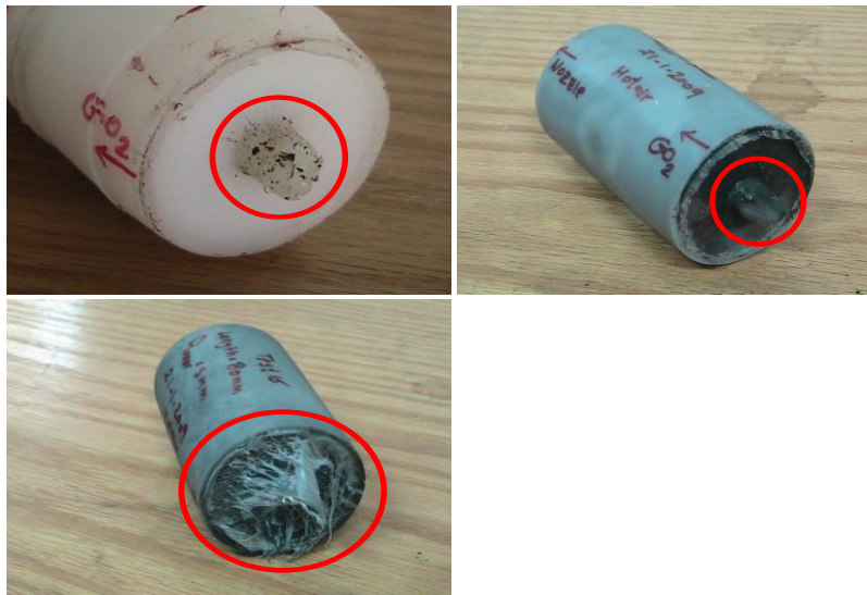
Fig. (3) Molten Fuel Material Moves Back to Block Injectors
