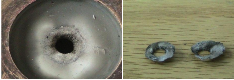
Fig.(10) Nozzle Throat as Affected by Al Particles
