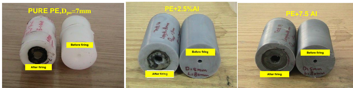
Fig. (2) PE Active Channel Port Before and After Firing
