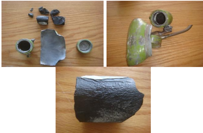
Fig. (7). Residual parts after firing test number 3
