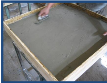
a) Casting the first layer of the base mortar
