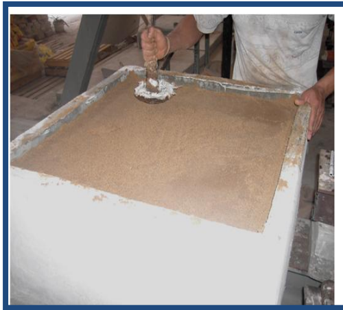
Fig. 6 Compacting the sand
