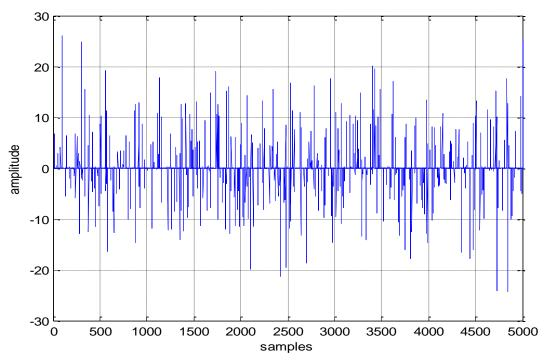
Figure (4): Time realization of highly impulsive (A = 0.1 and  $\Gamma = 0.5 \times 10^{-3}$ ) Middleton class A noise
