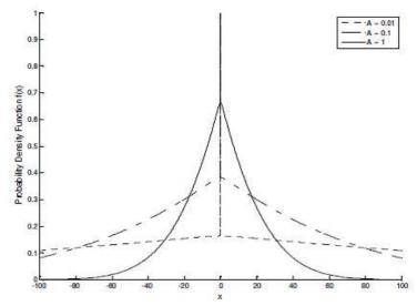
Figure (1): Probability density of the amplitude of Class-A noise with different values of A and  $\Gamma$ = 0.001 [16]
