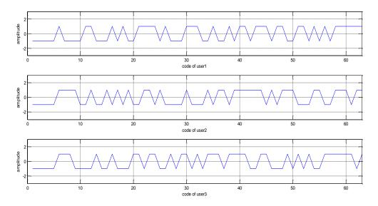
Figure (3): The original PN sequence waveforms of the 3 users
