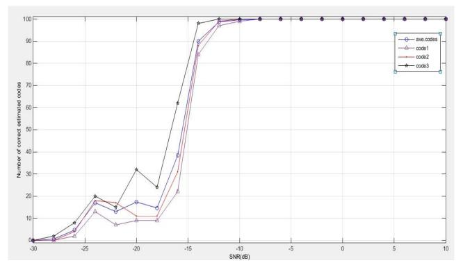
Figure 8: The number of correct estimated codes three codes at SNR=-13 dB
