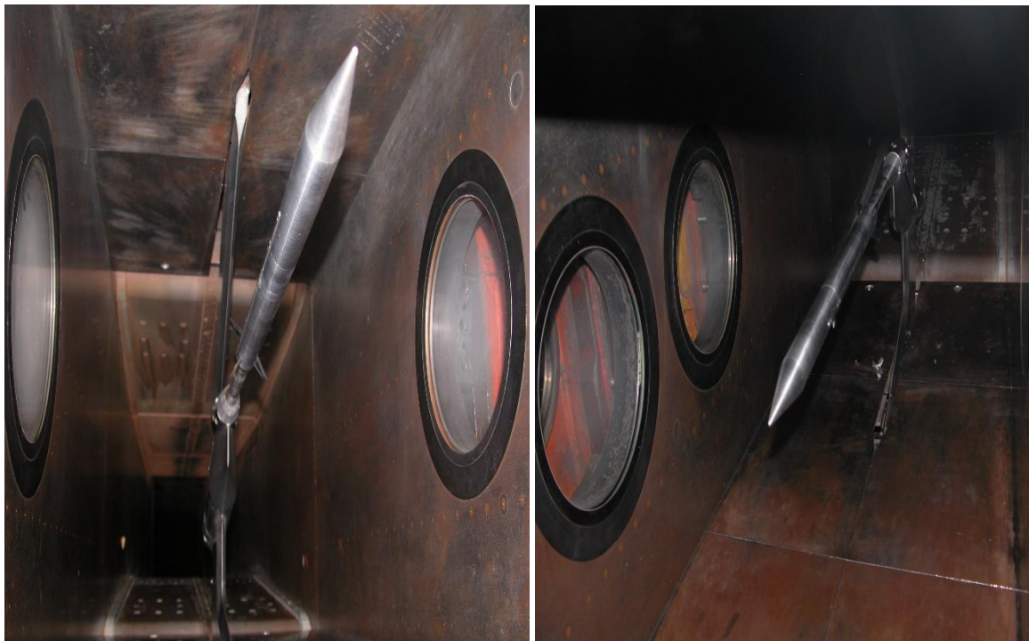
Fig. 2 model installation in the wind tunnel test section
