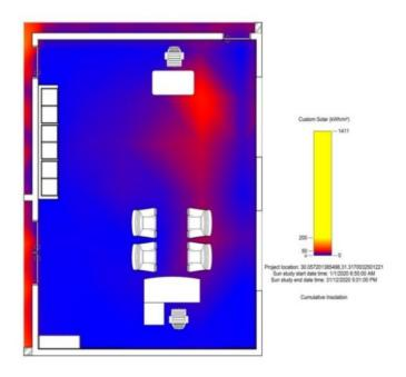
Figure 42: The heat load of the administrative space after using environmental treatments with values less than (55 kw/h/m2)
