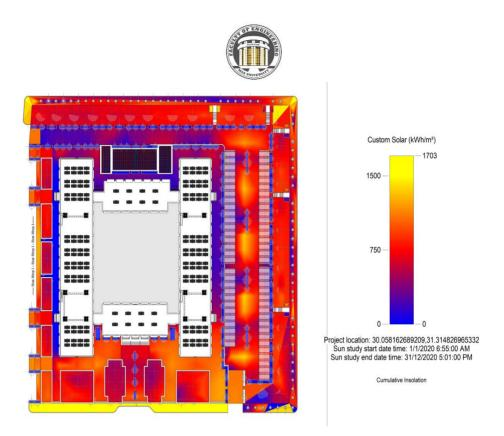
Figure 21: shows the heat load of the general site after using environmental treatments with values less than (850kw/h/m2).
