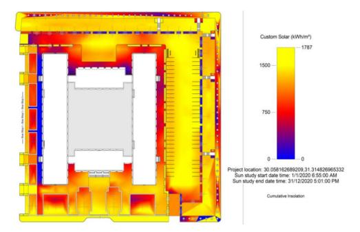
Figure 9: The researcher determined all the elements and factors of the general site, and measured the heat load using the simulation program (REVIT) for the general site (Fig.9), with values that exceeded (1500kw/h/m<sup>2</sup>).
