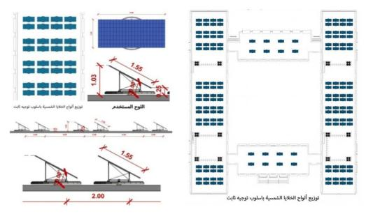
Figure 26: Shows distribution of photovoltaic matrices in a static routing fashion and open aggregation (proposed program).
