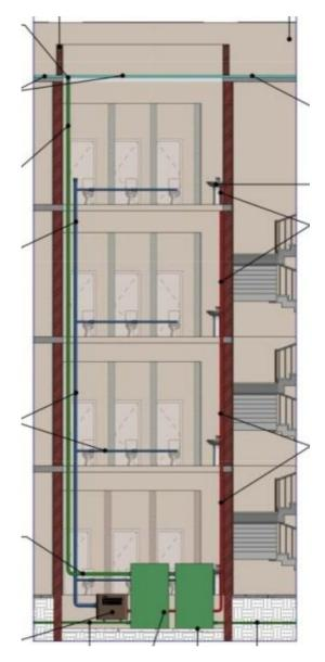
Fig (30): a vertical section of the building is passing through the bathrooms, showing the paths: collecting rainwater and draining rain (In green colour) and the path for collecting basin wastewater (In red colour) and directing it to the expulsion boxes in the bathrooms (In blue colour).
