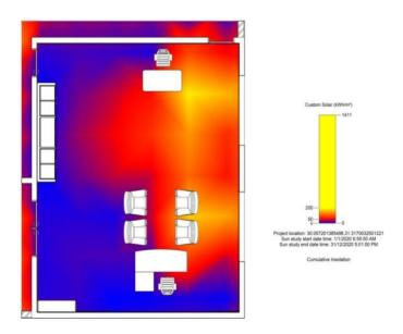
Figure 15: Shows the heat load of the administrative space, which reaches the highest value (250 kw/h/m2).
