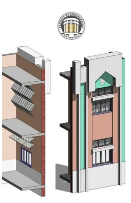
Figure 31: Wall curtains from reused and recycled materials to control the amount of natural light inside the spaces while maintaining air entry.
