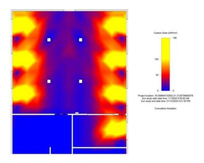
Figure 16: Shows the heat load of the classroom, which reaches the highest value (170 kw/h/m2).
