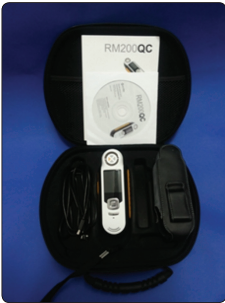
Fig. (5) Reflective spectrophotometer (X-Rite, model RM200QC, Neu-Isenburg, Germany).
