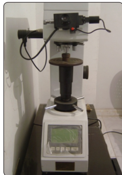
Fig. (2) The digital display Vickers micro-hardness tester.
