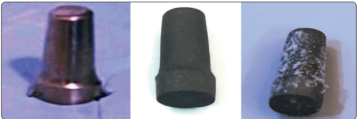
Fig. (2): From left to right: machined custom abutment, sand blasted custom abutment, and optical powder sprayed custom abutment.
