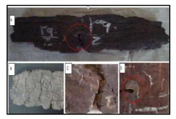
Fig 3 A: One of the Cheops pieces (piece no 390), B-C-D-Deterioration aspects and previous adhesive
