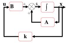
Fig. 1: State Feedback Closed Loop
