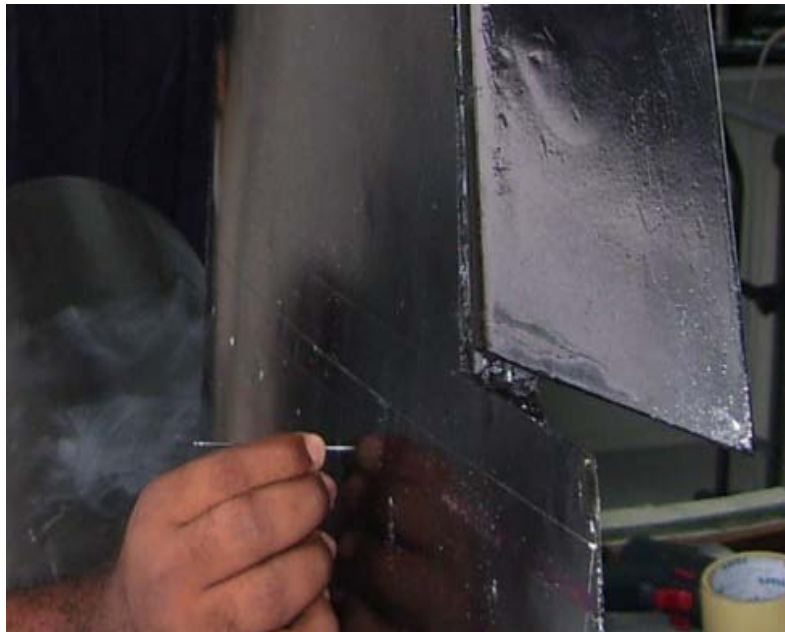
Fig. 8 Pressure tabs installation
