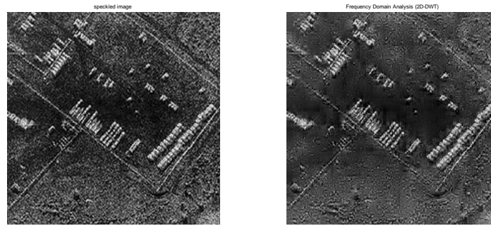
Fig. 2 (Left) Raw SAR Image, (right) Result of Frequency Domain Analysis
