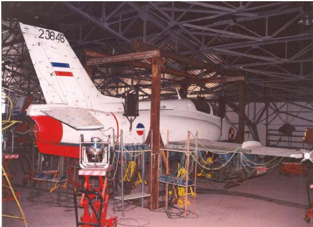
Figure 9 The ground vibration measurement and calibrations before flight test procedure[1]
