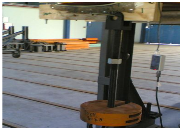
Fig. 10 Weights attached to wing
