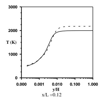
Fig. 8 Comparison between temperature distribution in premixed combustion for laminar and turbulent cases
