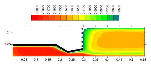
Fig. 18 Variation of CO2 mass fraction inside a combustion chamber equipped with nozzle.
