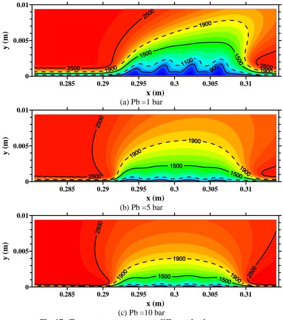
Fig. 17 Temperature contours at different back pressures
