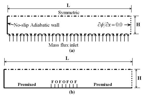
Fig. 1 The boundaries in case of (a) premixed combustion of propane in 2D duct, (b) methane combustion in dual premixed/diffusion configuration
