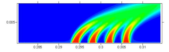
Fig. 7 Fuel concentration distribution along the combustion chamber
