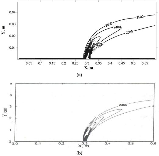
Fig. 5 Temperature distribution in case of diffusion flame using (a) the present model (b) the model of Chu and Yang [2]
