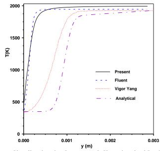
Fig. 4 Temperature distribution in the normal direction inside the reaction zone of propane premixed flame. Comparison between the present model, Vigor Yang model (Tseng et al. [1]) and Fluent code [9] as well as the analytical solution [4]
