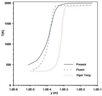
Fig. 3 Temperature distribution in the normal direction inside the reaction zone of propane premixed flame. Comparison between the present model, Vigor Yang model (Tseng et al. [1]) and Fluent code [9]
