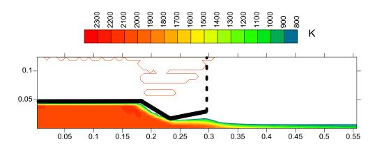
Fig. 19 Temperature distribution inside a combustion chamber equipped with nozzle
