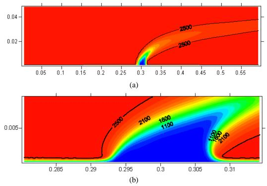
Fig. 6 Temperature distribution along the combustion chamber
