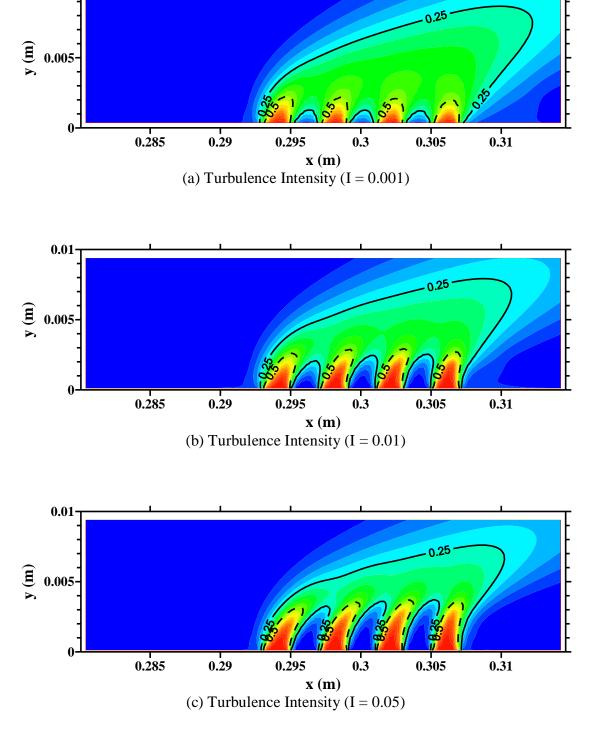
Fig. 9 Fuel concentration contours at different inlet turbulence intensities
