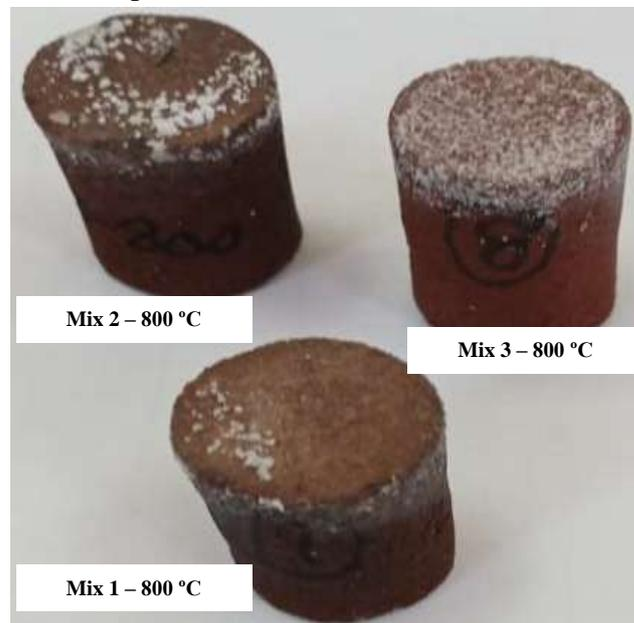
**Figure (9).** Results of efflourcense test for the fired briquettes.
