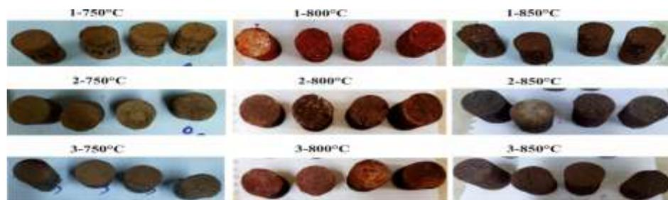
**Figure (10).** Color of briquettes of different mixes at different temperatures with different ratios of sand.
