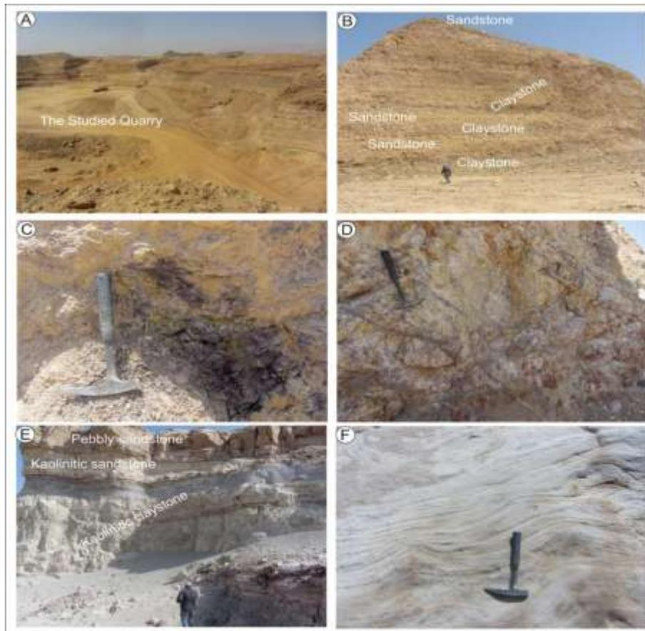
**Figure (3).** Field photographs showing, A- Open quarry in the Abu Darag area. B- Claystone with sandstone intercalations. C- Violet colored compacted clays. D- Pedogenic features (desiccation cracks, nodular fabrics and red mottling) in the compacted clays. E- White and grey kaolinitic clays in the upper part of the studied horizons. F- Thinly-laminated kaolinitic white sandstone.
