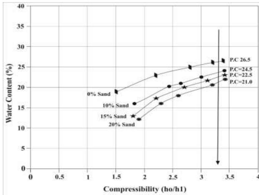
**Figure (6).** Results of plasticity test for the studied mixes containing different sand percentages.
