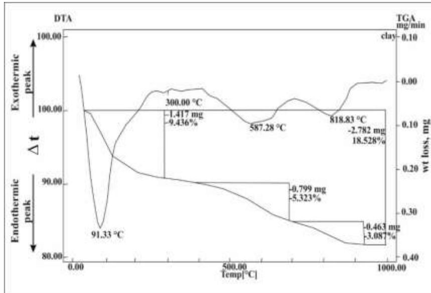
Figure (5). Results of thermal analyses (DTA-TGA) of the clay sample.
