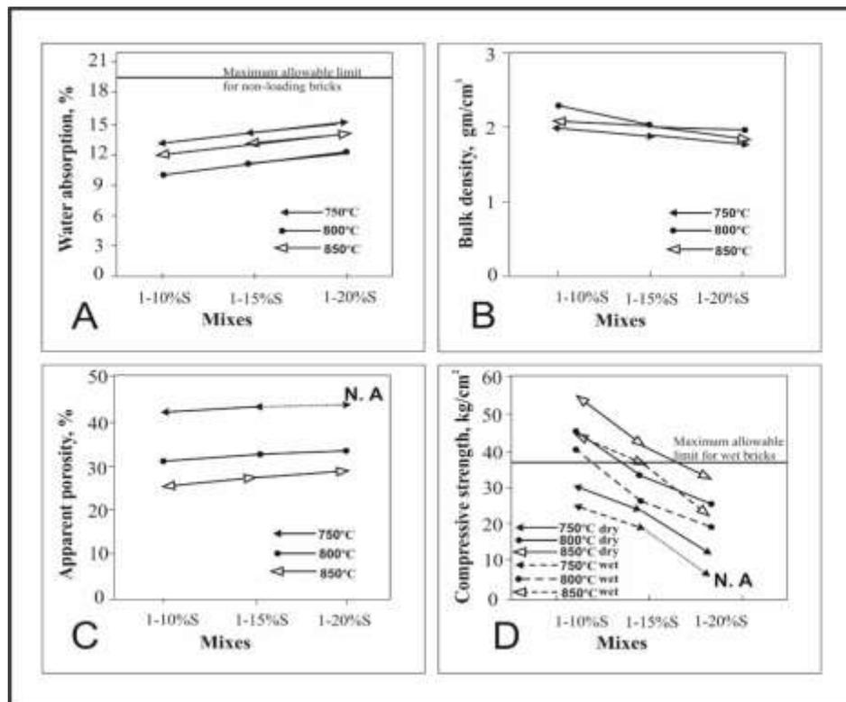
Figure (8). Physico-mechanical properties of the fired clay briquettes: (a) water absorption, (b) bulk density, (c) apparent porosity, (d) compressive strength.
