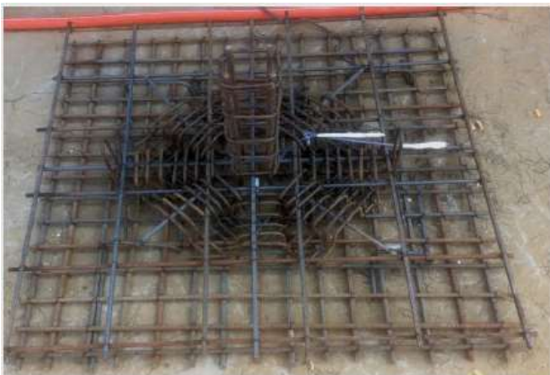
Figure 4: Layout of reinforcement details of Specimen S5.
