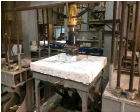
Figure 6: Loading test setup for the seven specimens.
