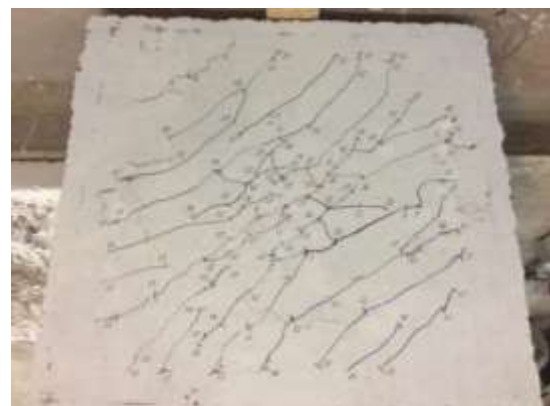
Figure 8: Cracking patterns for slab specimen S1.
