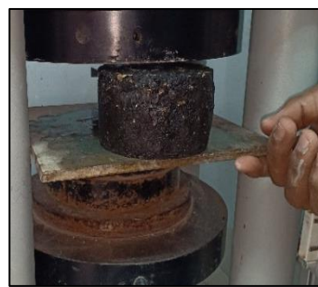
Fig. 6: Compressive Strength Test during Loading and at Failure.
