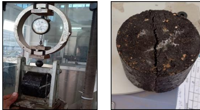
Fig. 4: Indirect Tensile Test during Loading and at Failure.
