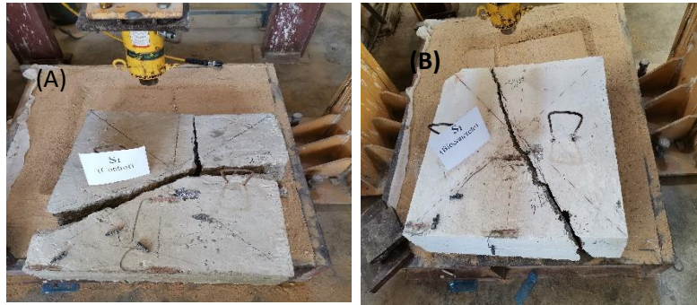
Fig.3: the crack failure pattern A.the control slab, B. the bio-concrete slab.
