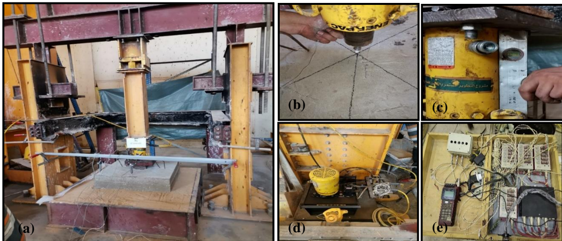
Fig.2: a. Frame setup with soil bed layer, auxiliary beam to support LVDTs transducers, b. position of central applied load, c. electrohydraulic Jack vertically leveled, d. electrohydraulic pump of the Jack, e. data logging machine.
