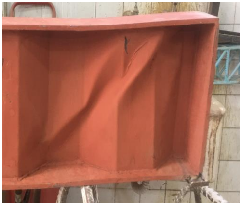
(a) Buckling mode for GCW1 Experimental versus FEM
