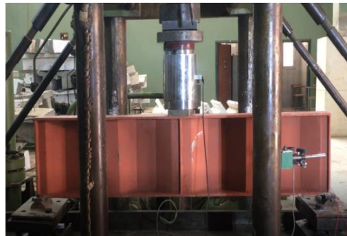
Fig. 9. Corrugated Girder under load test
