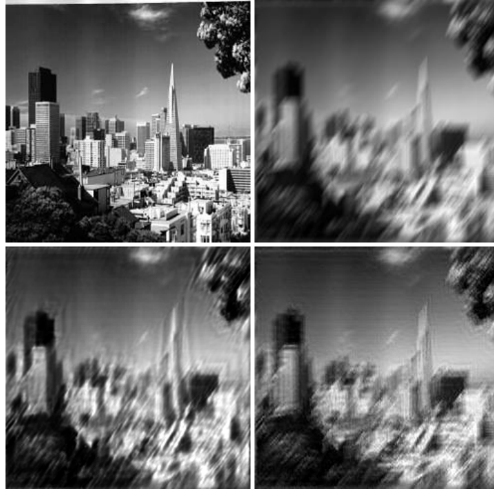
Figure 8: The top row represents the original san image, and the san image blurred with direction 55^\circ and large blur length 15. The left bottom is the result of Moghaddam [3] with direction 46^\circ and length 14, and the right bottom is our result with direction 65^\circ and length 7.
