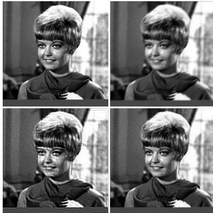
Figure 7: The top row represents the original girl image and the blurred girl image with direction 45° and length 5 respectively. The left bottom image is the result of Moghaddam [3] with direction 46° and length 7, and the right bottom is our result with direction 42° and length 5.
