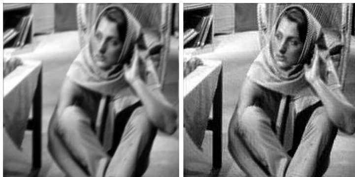
Figure 4: Left: The barb image blurred with direction 45^\circ and length 5. Right: The final result of GA with direction 44^\circ and length 5
