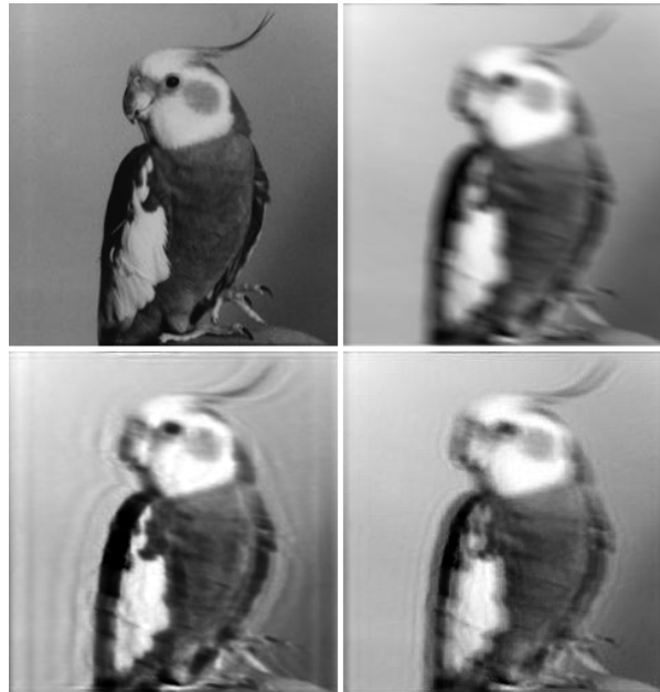
Figure 5: The top row represents the original bird image and the bird image blurred with direction 165^\circ and length 15, respectively. The left bottom represents the bird image restored with the correct parameters, direction 165^\circ and length 15. Notice the ringing effect. The image on the right bottom is the bird image chosen in the algorithm with direction 164^\circ and length 7.
