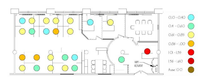
Figure 11: Average radio frequency measured at the chair of each working station.
