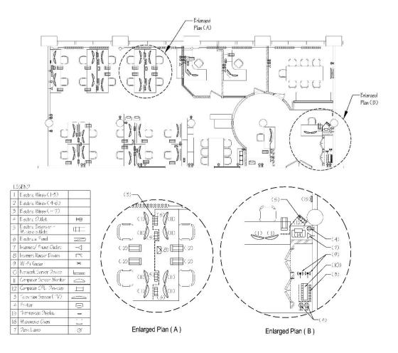
Figure 7: The space floor plan showing sources & devices emanating EMF/R.
