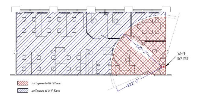
Figure 14: Recommended minimum distance of working desks from Wi-Fi routers.
