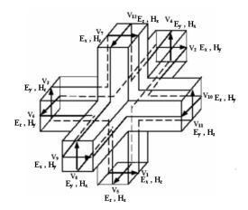
Fig. 1 Ports & field distribution in homogenous, lossless SCN
