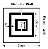
Fig. 2 A unit sample of the periodic SRR radar absorber
