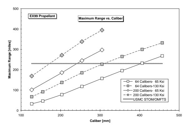
Figure 11: Maximum Range versus Gun Caliber for the Two Barrel Lengths and Breech Pressures
