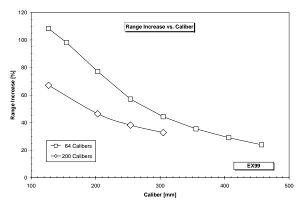
Figure 13: Percentage Range Increase Due to Increase in Breech Pressure versus Gun Caliber for the Two Barrel Lengths
