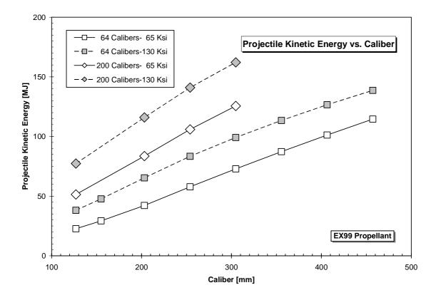
Figure 8: Projectile Kinetic Energy versus Gun Caliber for the Two Barrel Lengths and Breech Pressures
