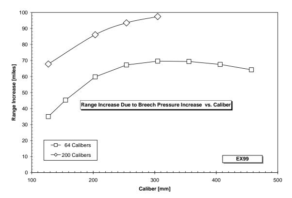
Figure 12: Range Increase Due to Breech Pressure Increase versus Gun Caliber for the Two Barrel Lengths
