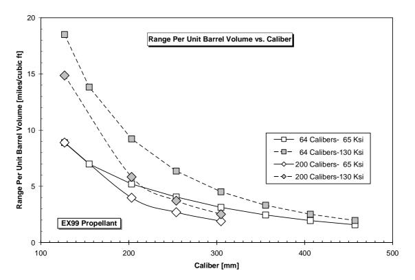
Figure 15: Range per Unit Barrel Volume versus Gun Caliber for the Two Barrel Lengths and Breech Pressures
