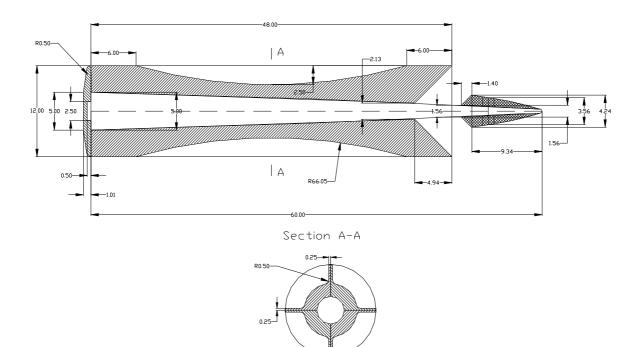
Figure 3: Design Drawing for the 12" Caliber Sabot
