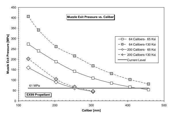
Figure 10: Muzzle Exit Pressure versus Gun Caliber for the Two Barrel Lengths and Breech Pressures
