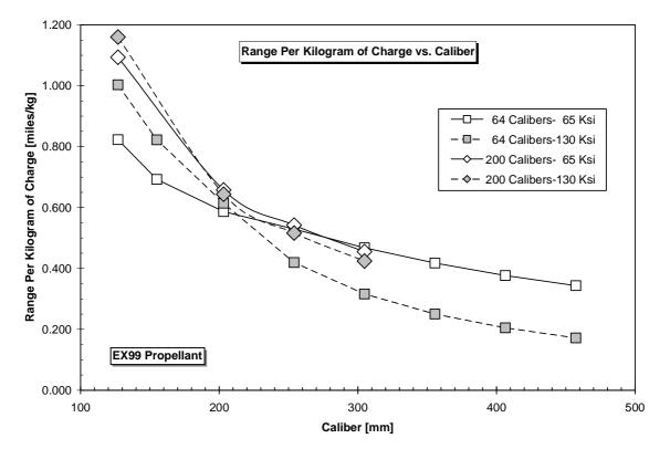
Figure 14: Range per Kilogram of Charge versus Gun Caliber for the Two Barrel Lengths and Breech Pressures
