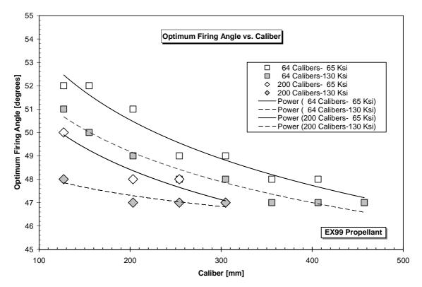
Figure 16: Optimum Firing Angle Curves versus Gun Caliber for the Two Barrel Lengths and Breech Pressures
