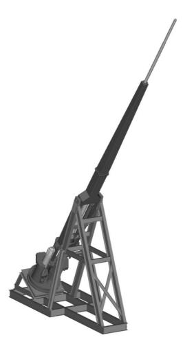
Figure 4: The Applied Ordnance Technology AOT or XLR Gun<sup>7,8</sup>; AOT Claims It Is Capable of Developing 200 Caliber Barrels
