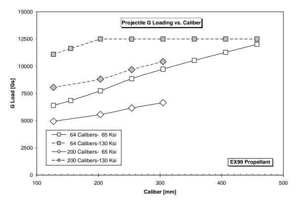
Figure 9: Projectile G Loading versus Gun Caliber for the Two Barrel Lengths and Breech Pressures
