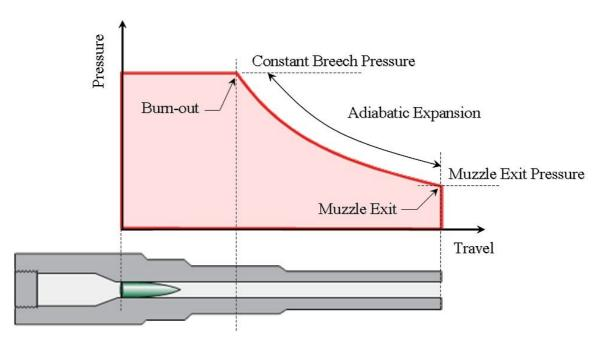
Figure 5: Schematic of the CONPRESS Model and the Pressure versus Travel Chart
