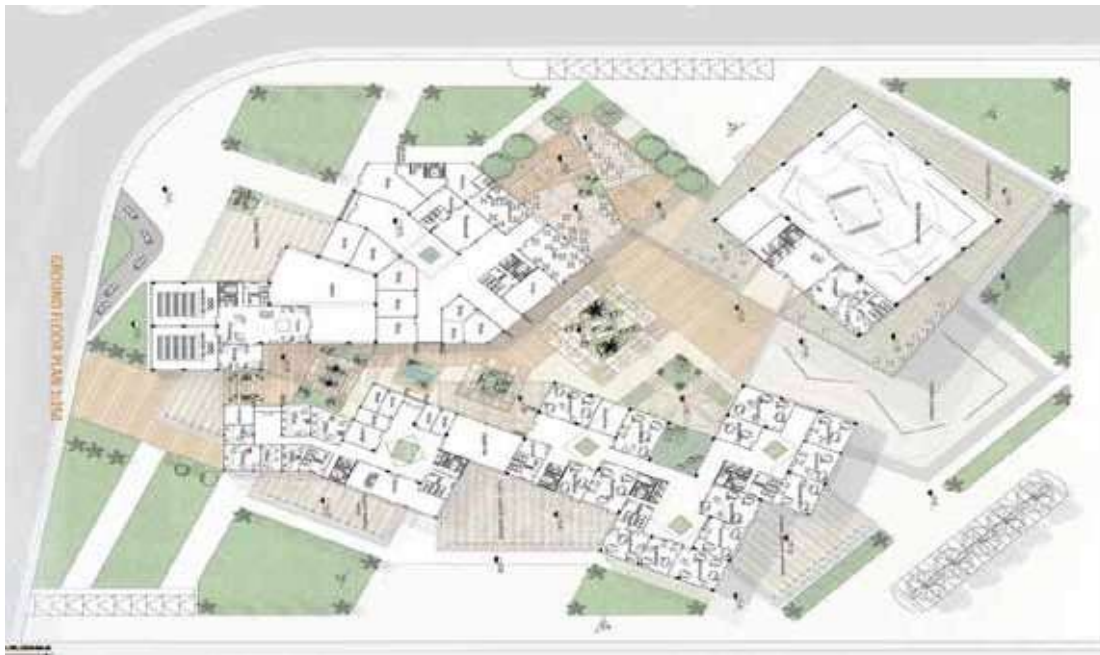
Fig. (54) The floor plan of the vocational training center which consists of the entrances, the commercial area, the main courtyard of the project, workshops and the main hall.
