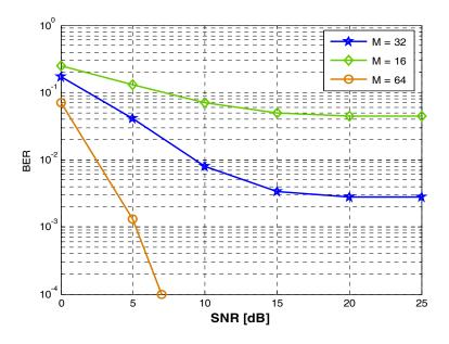
Fig. 7 BER performance versus variation of SNR, assuming equal SNR for all users, with following system parameters: Nt=1, Np=3, K=10, and Fd=8.
