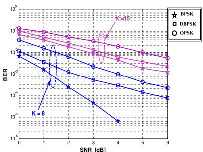
Fig. 11 BER performance versus variation SNR of the proposed system with Hamming coding, assuming equal SNR for all users, with following system parameters: Nt=2, Nr=1, G=30, M=32, and Fd=8.
