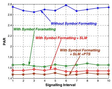
Fig. 5 PAR level at different signaling intervals with G=30, Fd=16, K=10, Nt=1, Nt=1, and M=32.
