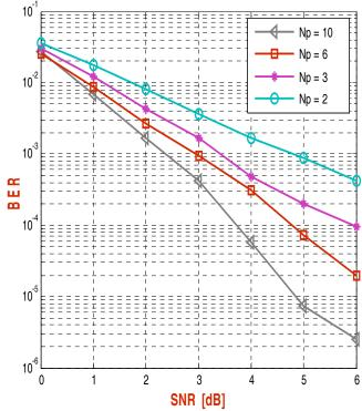
Fig. 9 BER performance versus variation SNR of the proposed system with Convolutional coding, assuming equal SNR for all users, with following system parameters: Nt=2, Nr=1, G=30, M=32, K=10, and Fd=8.
