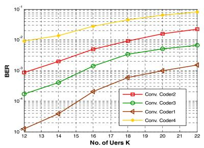
Fig. 12 BER performance versus variation in the number of users K with convolutional coding G=30, SNR=4 dB, Fd=8, Nt=2, Nr=1, and Np=3.
