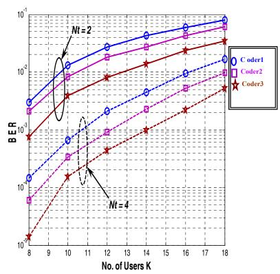
Fig. 17 BER performance versus variation in the number of users K with Hamming coding G=30, SNR=4 dB, Fd=8, Nt=2, Nr=1, and Np=3.
