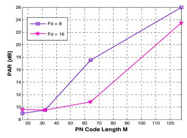
Fig. 6 PAR level versus variation in M value with Nt=1, Nr=1, G=10, and K=7.
