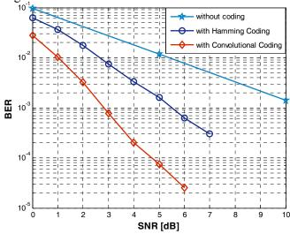
Fig. 8 BER performance versus variation of SNR, assuming equal SNR for all users, with following system parameters: Nt=2, Nr=1, Np=3, K=10, M=32, G=30, and Fd=8.
