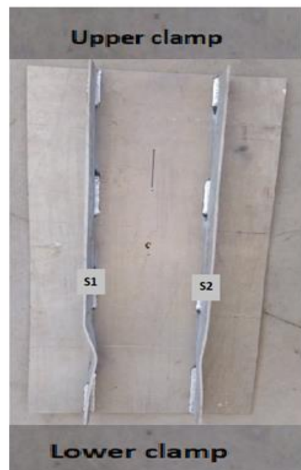
Figure 10: Collapse shape of specimen SP-LU
