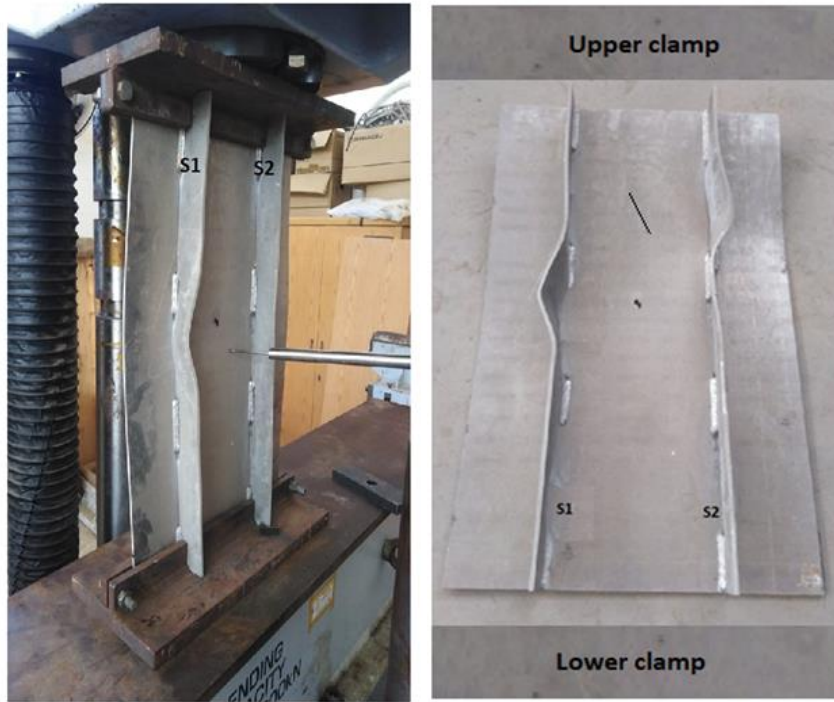
Figure 14: Collapse shape of specimen SP-AU during the test (left) and after (right).
