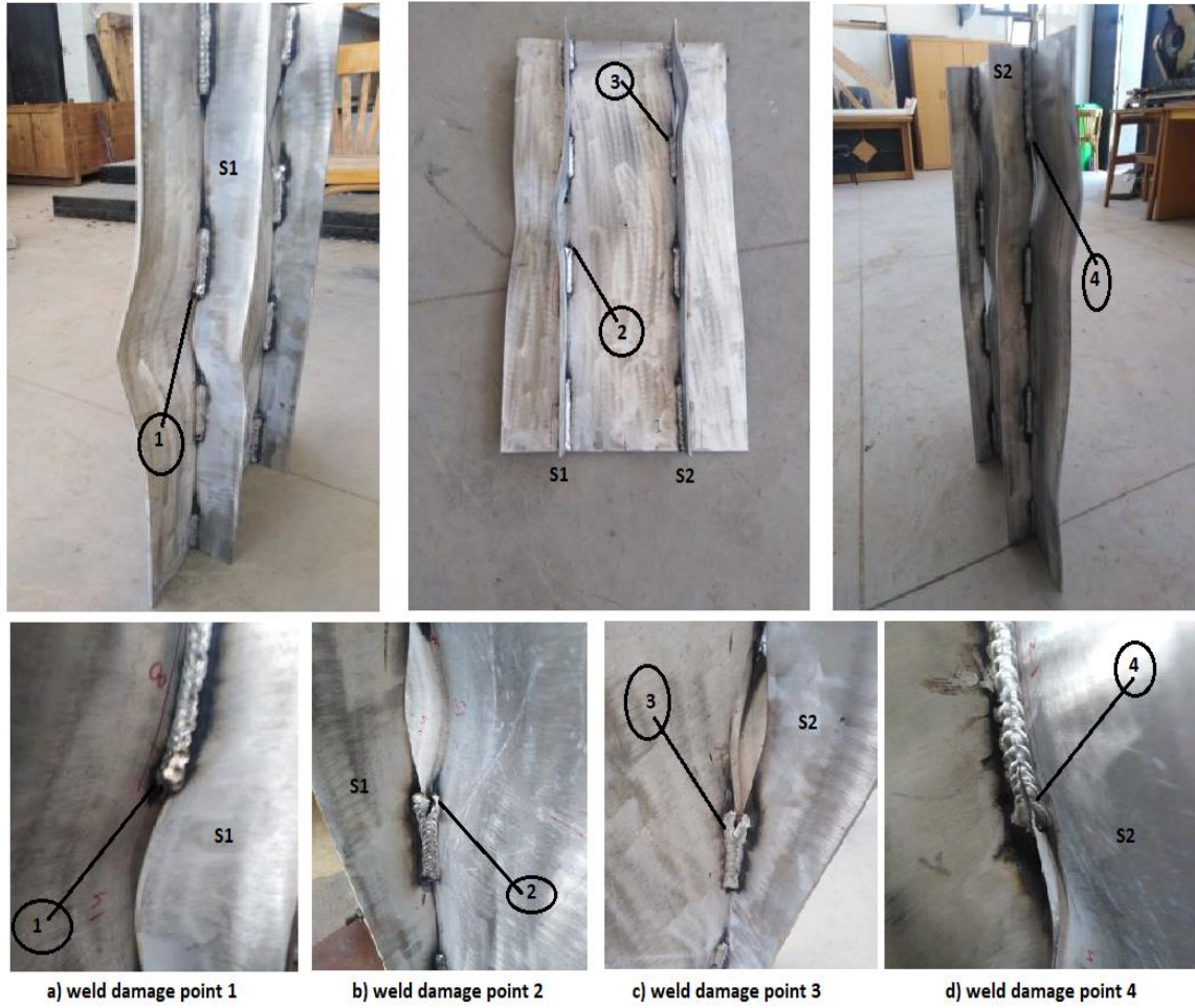
Figure 6: Collapse shape of the intact panel
