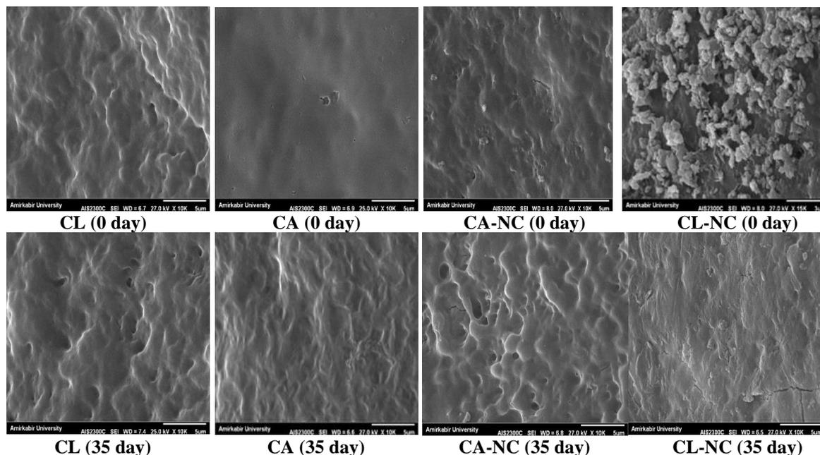
**Fig. 1.** Scanning electron microscopy images of eggshell outer surface at days 0 and 35 (Scale bar=5 $\mu$ m).
