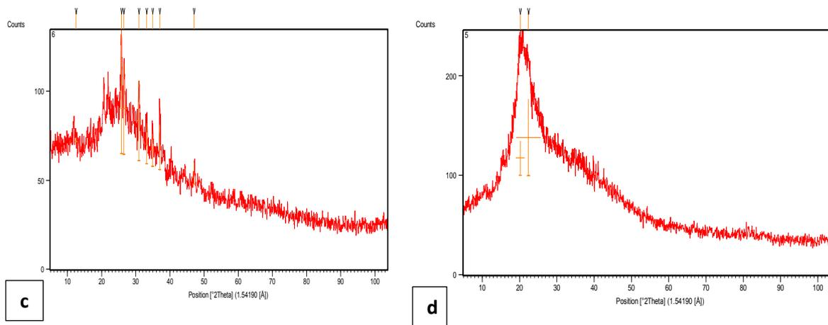
**Fig. 3** X-ray diffraction diagrams of CL (a), CA (b), CL-NC (c) and CA-NC (d) coated eggshell surfaces at day 35
