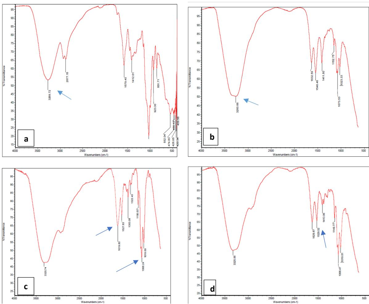
**Fig. 2.** Fourier Transform Infrared (FTIR) spectra of CL (a), CA (b), CL-NC (c) and CA-NC (d) coated eggshell surfaces at day 35
