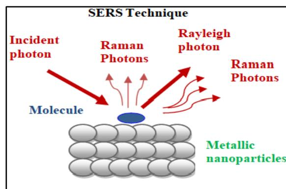
Fig. 3. Schematic diagram of the SERS effect.
