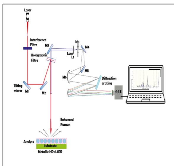
Fig. 4. Experimental setup for the SERS measurements.
