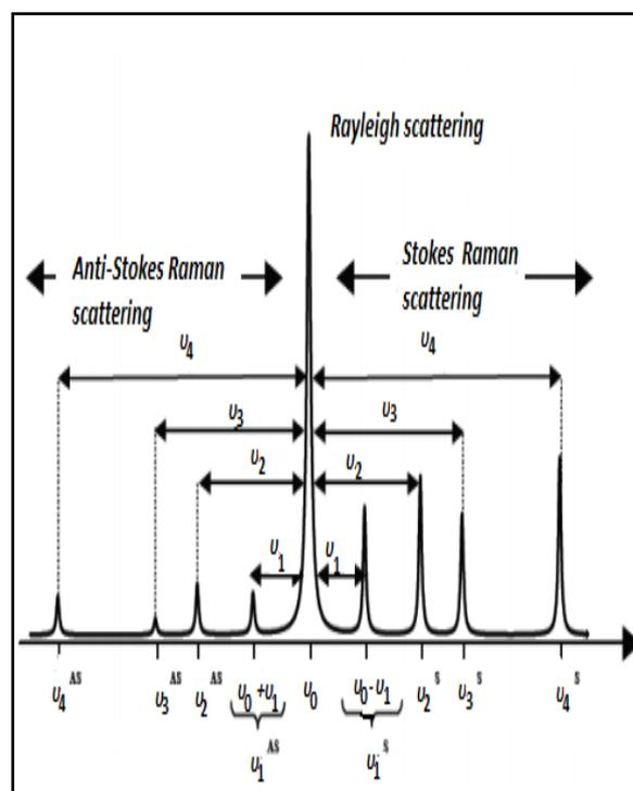
Fig. 1. Schematic representation of a Raman spectrum.
