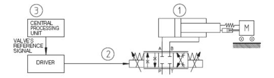
Fig.1 Automatic Open Loop Control of a Hydraulic Cylinder, Courtesy of Festo[1]
