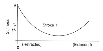
**Fig.6 Hydraulic Differential Cylinder Stiffness versus Stroke,** Courtesy of Vickers [2]
