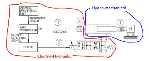
Fig.3 Electro-hydraulic and Hydro-mechanical Part of the System
