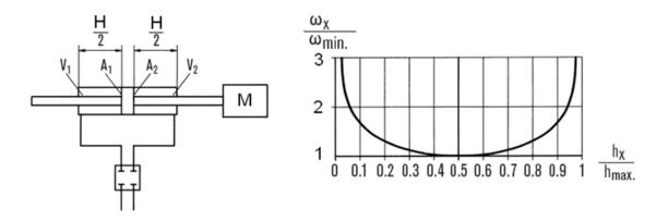
Fig.7 Hydraulic Synchronous Cylinder Stiffness versus Stroke, Courtesy of Bosh [3]
