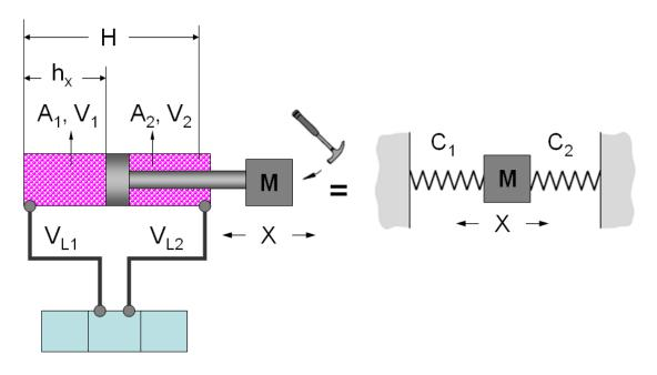
Fig.5 Simulating Hydraulic Cylinder Stiffness
