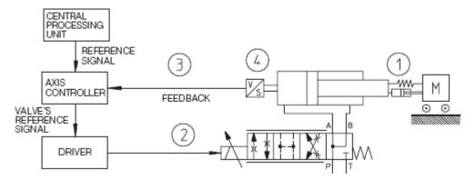
Fig.2 Automatic Closed Loop Control of a Hydraulic Cylinder, Courtesy of Festo[1]
