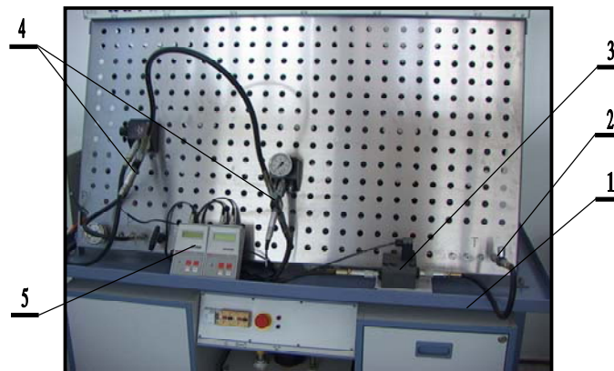
Fig. 4. Test rig of hydraulic losses measurement
